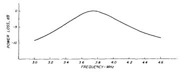
fig, 16. Calculated equivalent loss in the balancing resistor for the turnstile antenna driven by a Wilkinson hybrid.
